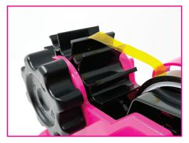
Stick the heat tape to the underside of one of the auto cut reel sectional flaps.
