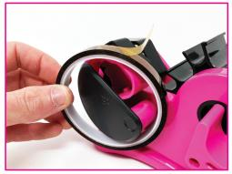
Place the heat tape roll onto the standard dispenser wheel.
